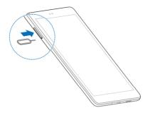
Pull out the card tray and place the nano-SIM card and the optional microSDXC card on the tray, as shown. Carefully slide the tray back into place.
